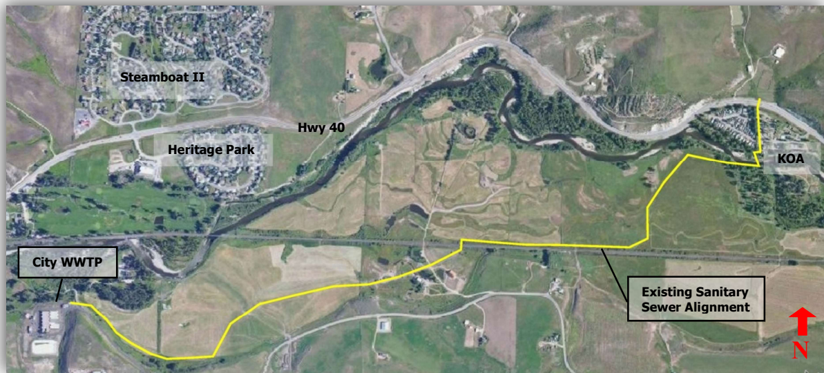
Figure 1 - Sanitary Sewer Serving West Steamboat
