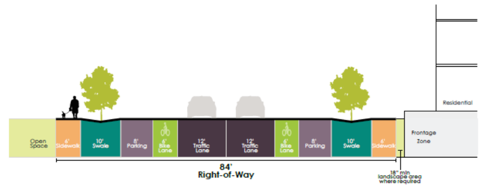
CONNECTOR RESIDENTIAL 2 CITY STREET STANDARDS: CONNECTOR - PARKING ON BOTH SIDES
